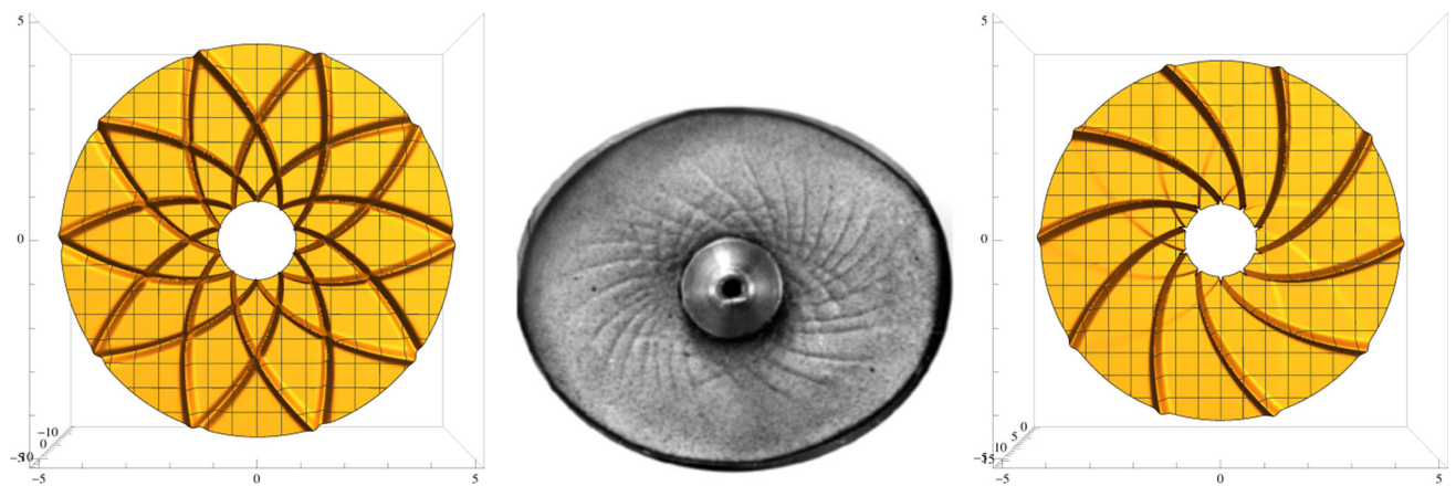
Fig. 6 The \sigma_{r\theta} -chain solutions (left) for the fabric tensor measured from Fig. 4 of [26]. For a clear comparison with the experimentally observed Mandala-like slip lines (centre, courtesy of Bobryakov and Revuzhenko [26]), only ten chain pairs are shown. The rotation in the
